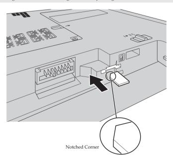
**6** Put the battery back in place. Turn the computer over and reconnect the cables.
